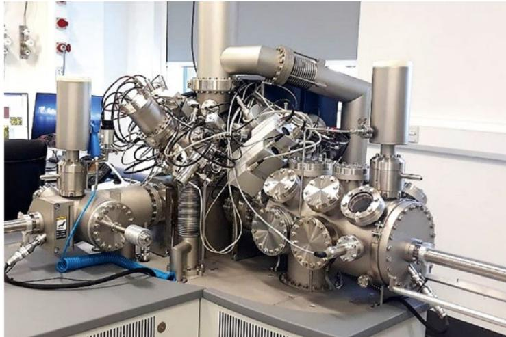
Time-of-Flight Secondary Ion Mass Spectrometry (ToF-SIMS) equipment
