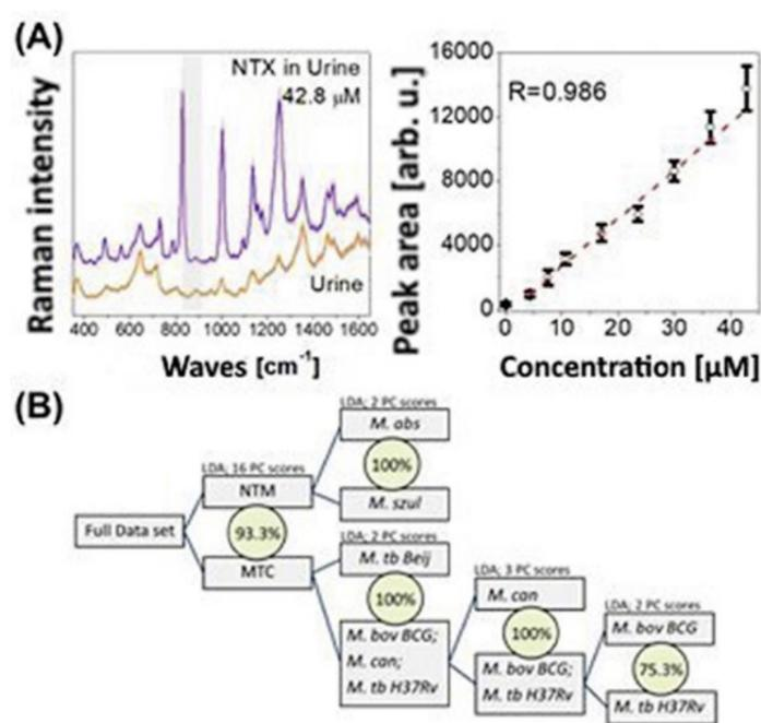
Figure 2: (A) The SERS spectrum of NTX in human urine and the background-SERS spectrum of pure human urine (measured with the *Lab-on-a-Chip* SERS setup). Linear dependency of the measurement signal (peak area of the marked Raman-band) and the concentration of an NTX-spiked urine sample. (B) Identification of mycobacteria: structure and parameter of the identification tree of the chemometric model based on the database that was created.
