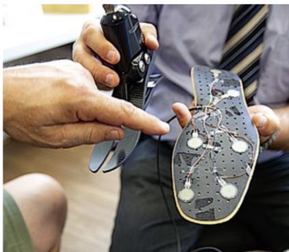
Six sensors were fitted to the foot sole of the lightweight prostheses and these were then linked to stimulators inside the shaft where the amputee's stump sits.
