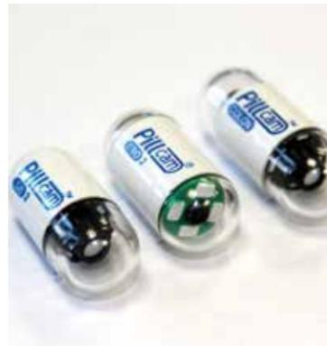
The capsule contains a minuscule camera that can impressively capture up to 35 images per second
