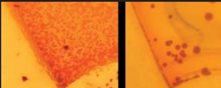
A synthetic surface coated with biocide. Colonies of Staphylococcus aureus are coloured red. The untreated control sample (left) shows uninhibited cell growth. The coated sample (right) shows a 100 times reduction in the number of germs. The test was carried out according to guidelines for spray tests.
