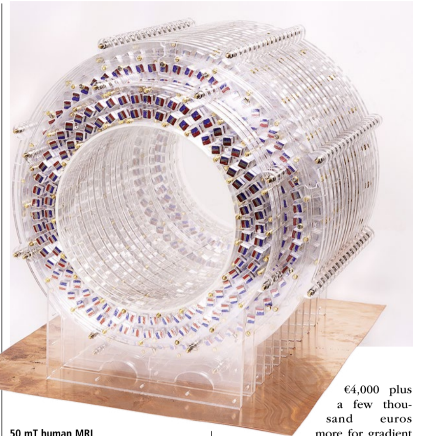
50 mT human MRI system developed in the Department of Radiology at the Leiden University Medical Center.
