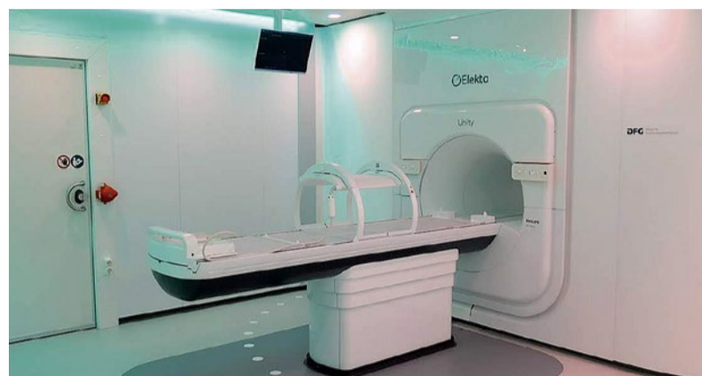
MR-Linac (Unity, Elekta AB, Sweden) at the University of Tübingen (DFG ZI 736/2-1): a hybrid system combining a 1.5-T MRI scanner with a 7-MV linear accelerator for online adaptive MR-guided radiotherapy
