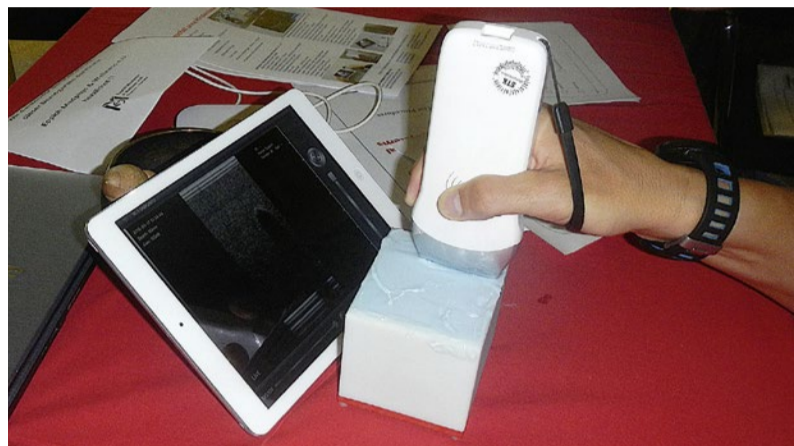
Wireless transducer (LA) being used in a training session on the recognition of artefacts (phantom). The real-time ultrasound images (b-mode) are transmitted via WiFi to a tablet (iPad/Android)
