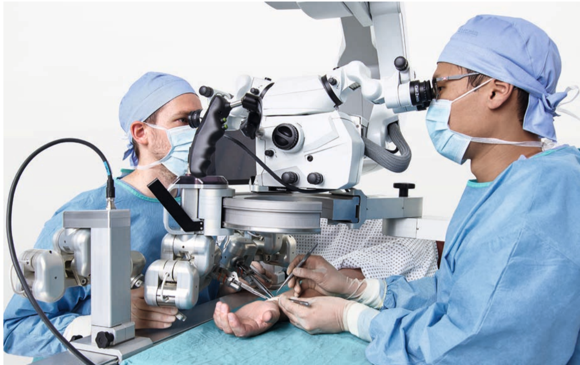
MUSA, the world's first clinically available CE marked microsurgery robot © Microsure BV
