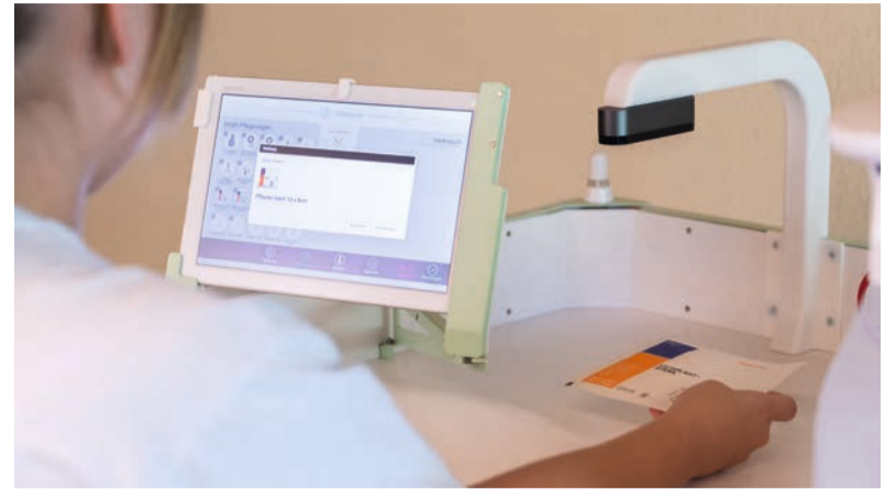
Sensors scan each item taken from the shelves to facilitate stock management. © Fraunhofer IPA
