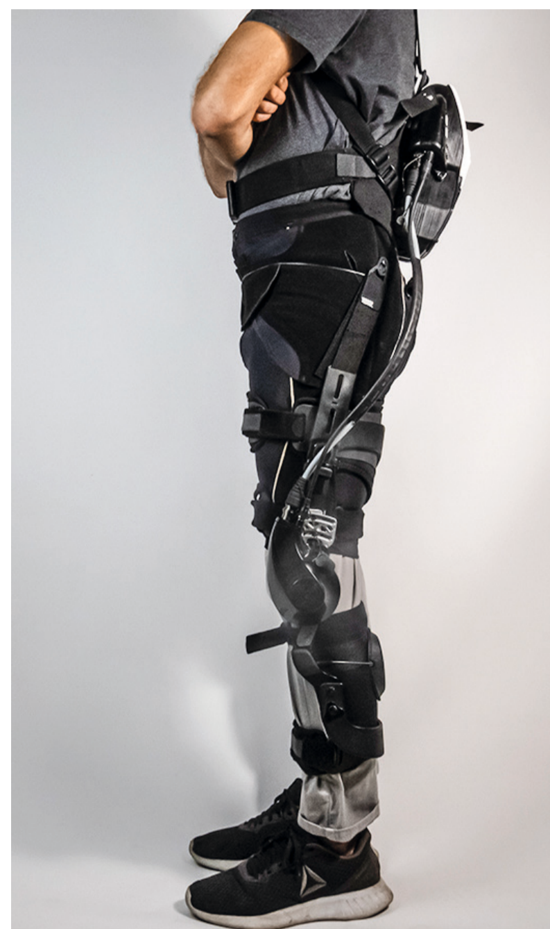
Knee exoskeleton that provides both flexion and extension assistance during walking, to improve weight-bearing ability. © ICRA
