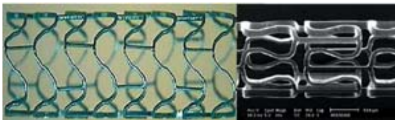
Absorbable metal stent (from Biotronik) after expansion (left panel) and in electron microscopy magnification (right panel)
